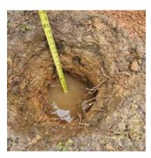
3. Monitor water depth in 4-8 hour intervals. Take a photo at each check. Record date and the time when hole is empty. Take a photo of the hole when empty or at 36 hours.
